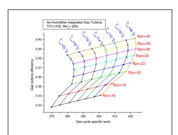
Fig 8. A design monogram of plant efficiency versus plant specific work in an AHIGT for different TIT and and drop in temperature of air in the humidifier
