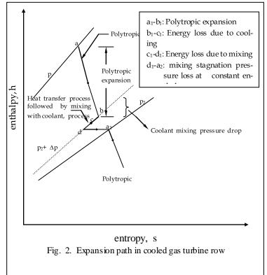
Fig. 2 gives the details of expansion process for a cooled turbine stage. Process  $b_1$ - $c_1$  in Fig. 2 depicts cooling due to heat transfer between hot gas and coolant, which takes place at constant pressure line due to which exergy decreases, while process  $c_1$ - $d_1$  depicts drop in temperature due to mixing of coolant with gas which
