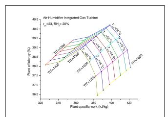
Fig 7. A design monogram of efficiency versus specific work in an AHIGT for different TIT and drop in temperature of air in the humidifier due to rise in ambient temperature
