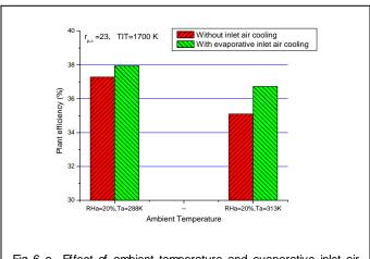
Fig 6 a. Effect of ambient temperature and evaporative inlet air cooling on plant efficiency
