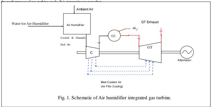
the mass of coolant required for gas turbine blade cooling is a function of inlet air temperature and reduces with increase in temperature drop.
